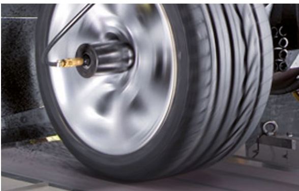
©IABG mbH - IABG flat track tire test stand Flat-Trac® III CT Munich /Ottobrunn
